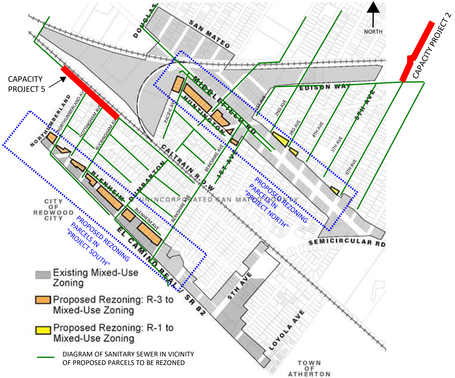
FIGURE 2 - FAIR OAKS SEWER MAINTENANCE DISTRICT CAPACITY PROJECTS
